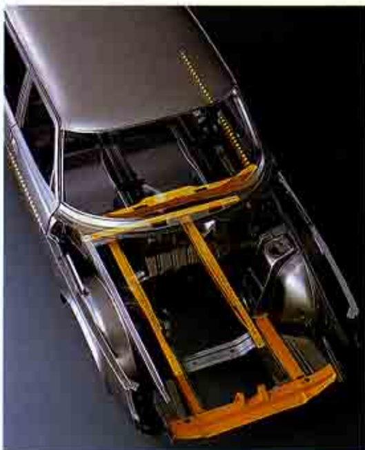
Crash members Members which transmit forces from a frontal collision to the wheel housings and arrest rearward movement of the engine.
